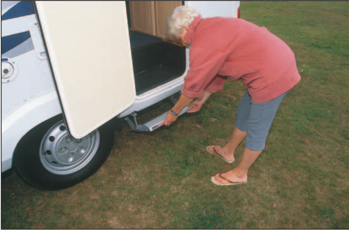
Manually-operated step cuts down on manufacturing costs but an electric one would be better. A warning buzzer sounds in the cab if the step is left out.
