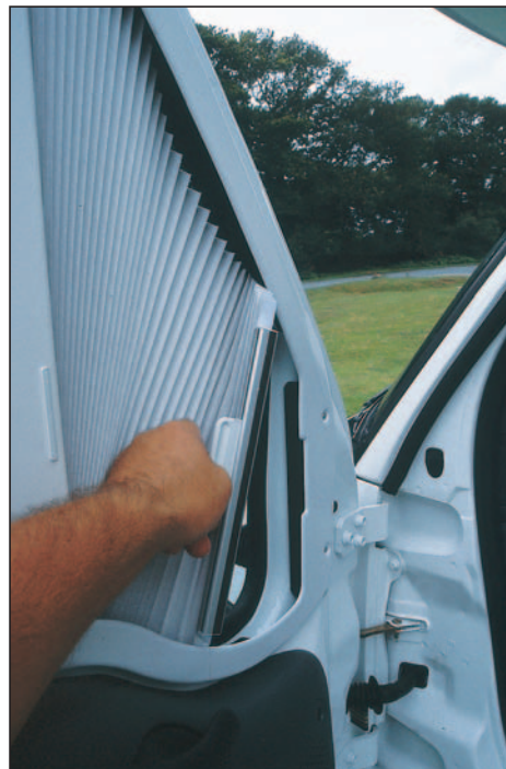
Prototype cab door blinds are very easy to operate and secure by means of a magnetic strip. On the driver's side ► the wing mirror is partially obscured by the cassette holder.
