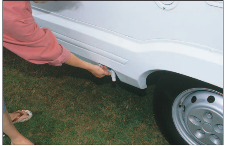
The drains for the fresh and waste water tanks are located on the rear and offside in front of the rear wheels. They drain freely and are easy to get to.
