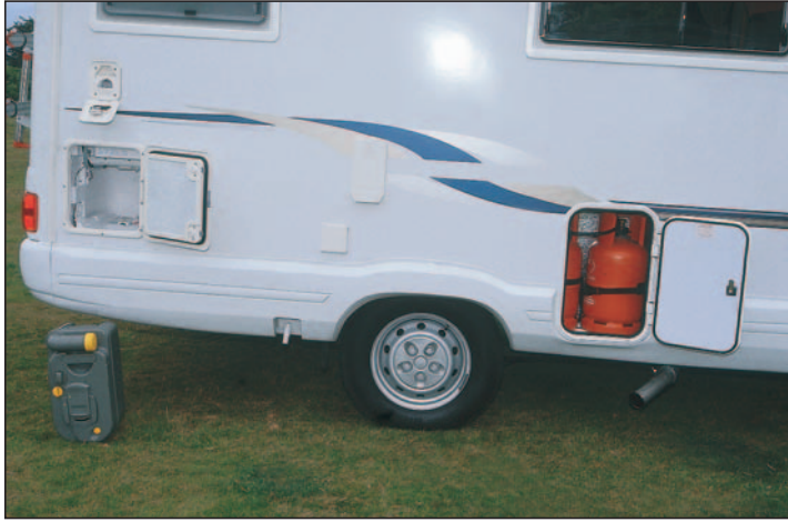
Filler for toilet flush tank is above the cassette access door. Gas compartment holds two 6/7kg cylinders.
