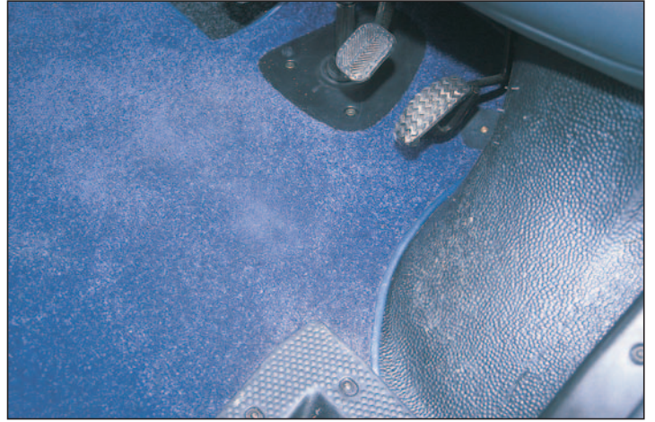
Cab carpet is not removable and after only a few hundred miles marks where the accelerator foot meets the floor were beginning to show.
