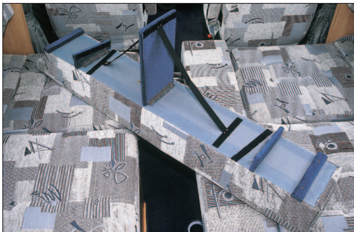
The legs supporting the bed's centre section displayed a tendency to 'cave in'.
