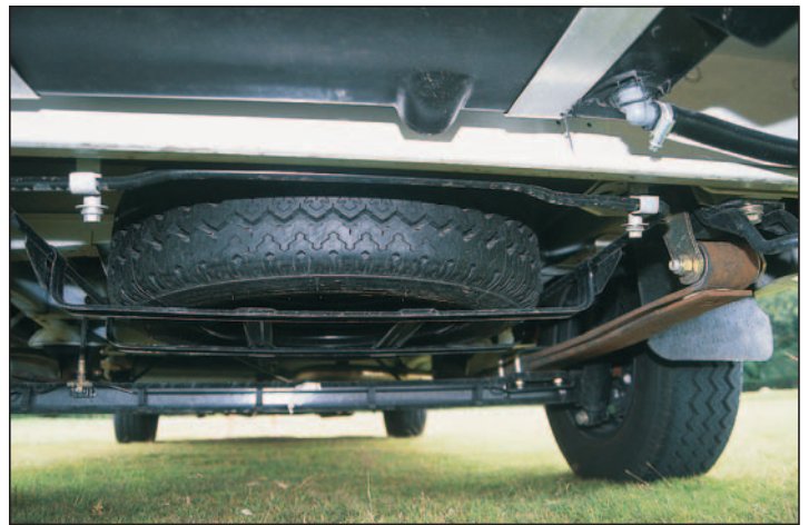
The spare wheel is located behind the waste tank and is difficult to access.
