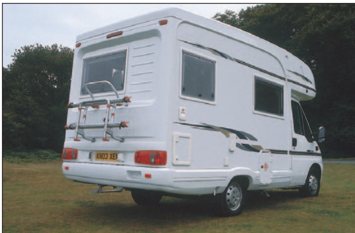
Top bar of the cycle rack partially obscures the driver's rearward view.
